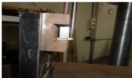
Shear bond strength test of the samples (Fig:3)
