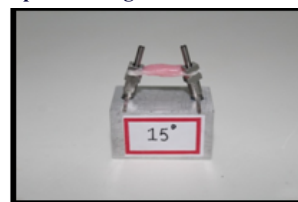
Splinting of 15° implant analogues with Autopolymerizing resin.
