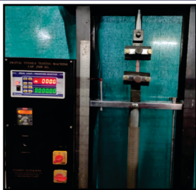
FIG 7- Specimens ready for testing in Universal Testing Machine.
