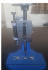
II. Testing of samples using Vicats apparatus after exposing to heat
