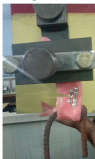
Fig. 4. Set-up of S.S. mini plate and PMMA block for tensile strength.
