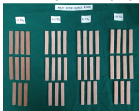
Fig 3: PMMA specimens reinforced with different concentrations of \text{TiO}_2 nanoparticles
