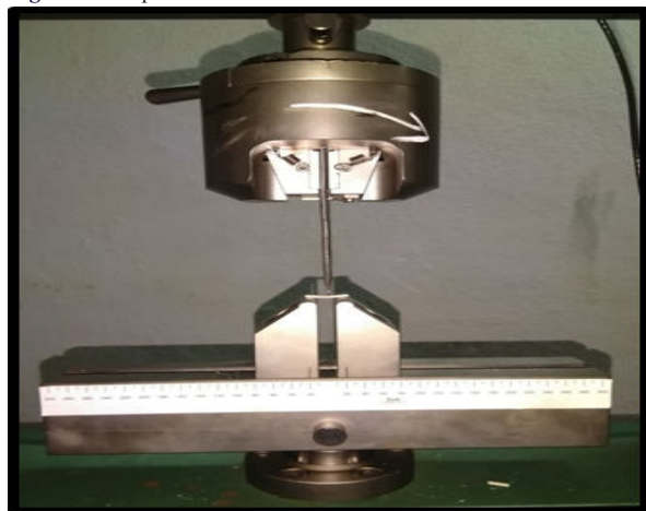
Figure 3: Testing Of Samples Under Universal Testing Machine
