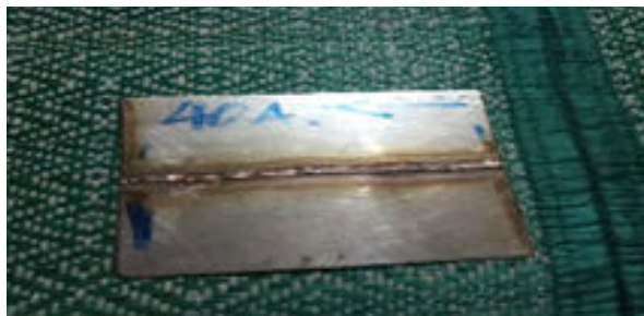
Figure 2. SS 304 plate connection number 1
