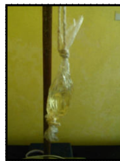
figure 3: Dialysis tubing cellulose membrane with AZM gel
