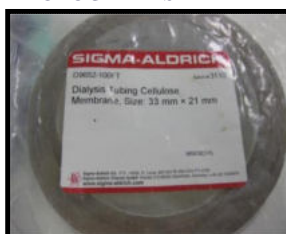
figure 1: Dialysis tubing cellulose membrane.
