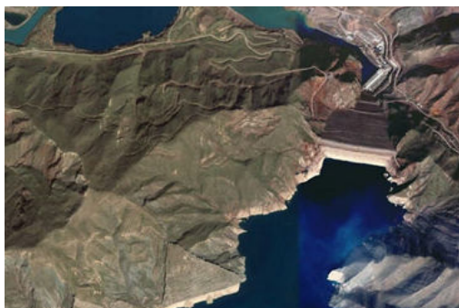
Figure 1: The Nurek Dam, located in Tajikistan in 304 m zoned earth fill, built between 1961 and 1980 (source Google Earth)
