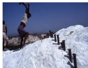
Photograph 1: Manual method of marble block recovery
