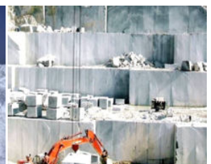
Photograph 2: Mechanize method of marble block recovery
