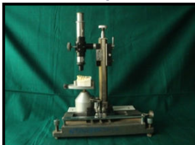
Figure 7: Linear distance measured using travelling microscope
