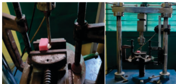
Figure 1:- placement of specimen under universal testing machine
