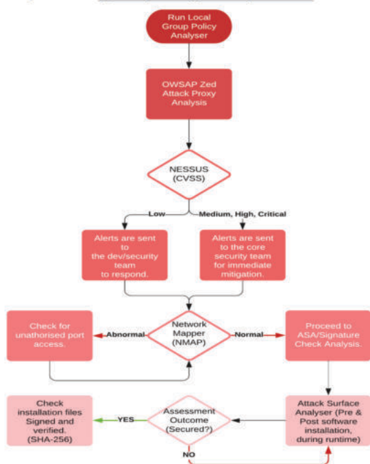
Fig 2. Proposed Cybersecurity Analysis Algorithm for Calibration Software
