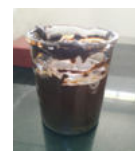
Figure 1.2: After mixing with sodium carbonate at 16000ppm emulsion is formed
