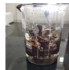
Figure 1.1: (without mixing sodium carbonate) no emulsion formed
