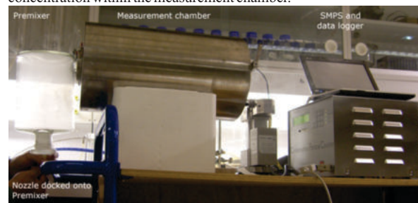
Fig. 2 Exposure system consisting of a 2.5 L premixer made of glass and a 22 L main steel chamber. The particle scanner is attached at the proximal end of the main measurement chamber.
