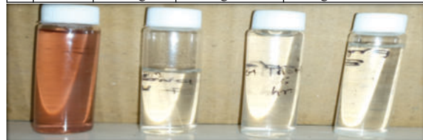
Fig.4 : changes of real textile industrial waste water colour with time using anatase TiO 2 and UV radiation
