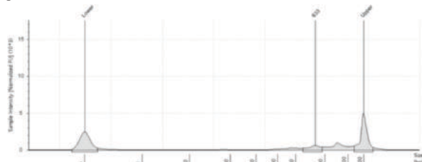
Figure 2. Analysis by Agilent TapeStation system Electropherogram of sample intensity (in fluorescence units, FU) for amplicon analysed by Agilent TapeStation High Sensitivity DNA assay. (Lower: lower marker; Upper: upper marker).
