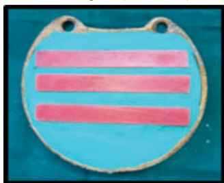
Figure 1: Wax pattern fabrication
