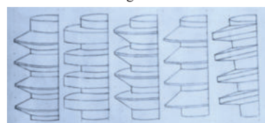
Figure 5: Different Thread Shapes : A. V Shape B. Square Shape C. Buttress D. Reverse Buttress E. Spiral Shape
