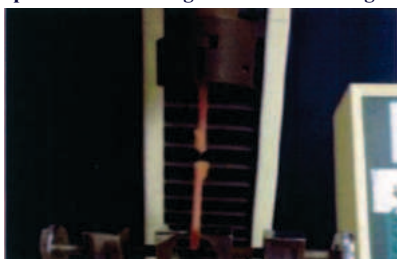
Figure 10 – Specimen After Bond Failure
