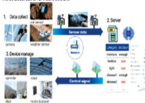
Figure 2: Architecture of grid-based communication network for large scale cloud smart farms
