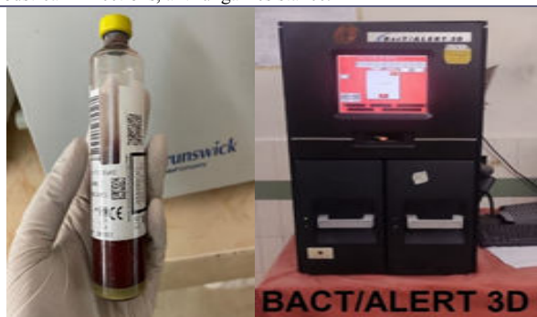
Figure 2: BactAlert bottle and machine
