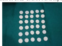
Figure 1: Finished Specimens Of Compression Molded Self-cure Pmma
