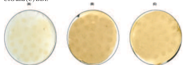
Fig. 2 Image of the filters after collection of mainstream emission of single unit of (A) THS, (B) CIG and (C) BDI.
