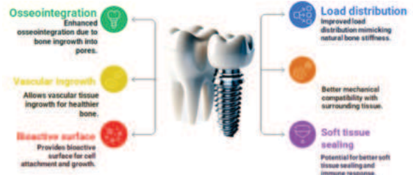
Figure 2: Advantages of Porous Titanium Implants
