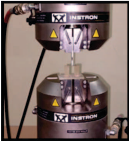
Figure 9 – Metal-ceramic Sample Placed In Universal Testing Machine For 3 Point Bend Test
