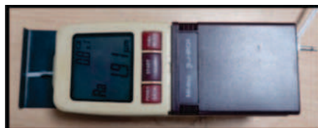
Figure 6 - Sample Is Placed On The Contact Profilometer For Checking Surface Roughness
