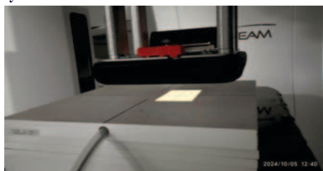
Figure 3: Alignment of the Phantom After Moving the Table 3cm Laterally From the Isocentre
