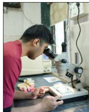
Fig 4: Internal fit assessment using stereomicroscope
