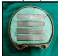
Fig1: Stainless steel mould for tensile strength
