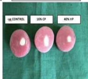
Fig 7: Representative sample of each group after embedding in cold cure acrylic resin
