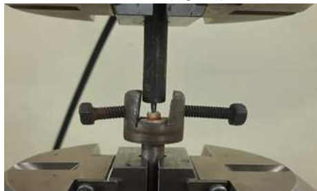
Figure 2: Fracture resistance testing using universal testing machine
