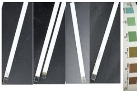
Figure 4. Hydrolysis of Tapioca Starch by \alpha -Amylase: Glucose strip test indicating a low glucose production following enzymatic digestion of tapioca starch.
