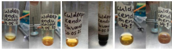
Figure 2 - Kendu leaf extract phytochemical analysis – A: Alkaloid test, B: Flavonoid test, C: Phenol test.
