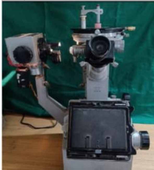
Figure 2. Vickers hardness machine. Post treatment microhardness evaluation (T1)
