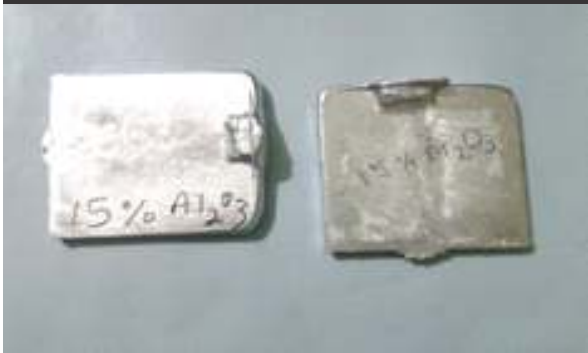
Fig. 4 AMMC with 15% aluminium oxide
