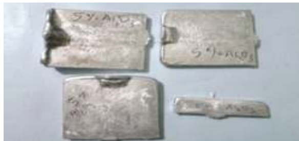
Fig.2 AMMC with 5% aluminium oxide
