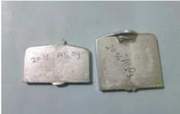
Fig. 5 AMMC with 20% aluminium oxide
