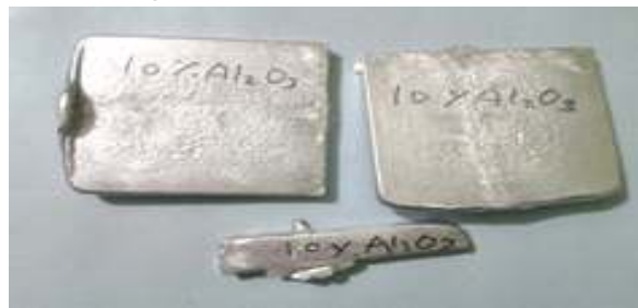
Fig. 3 AMMC with 10% aluminium oxide
