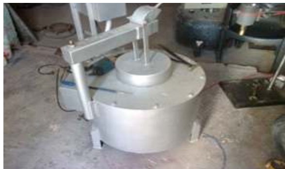
Fig.1 Stir casting set up
