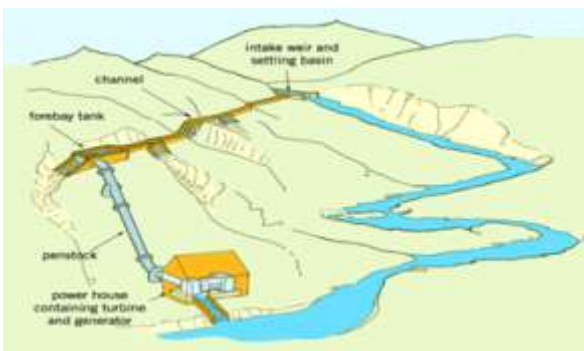
Fig.3. Schematic of typical run of river SHP Scheme
