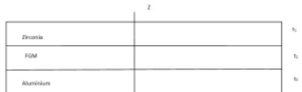
Figure 1. Zirconia/FGM/ Aluminum composite FGM plate.
