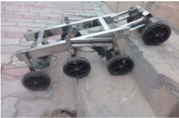
Figure 11.1: Stair climbing of robot
