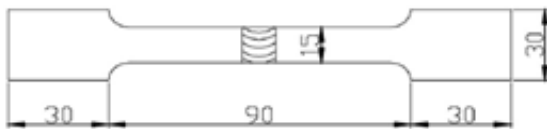
Figure 3 Dimensions of Tensile Specimen
