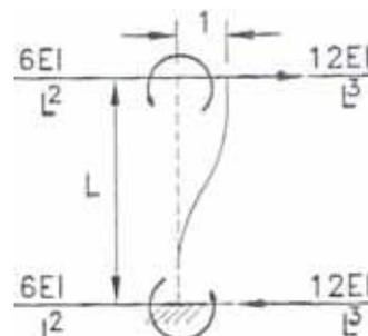
Fig. 2 Forces and moments generated at the ends due to unit displacement.
