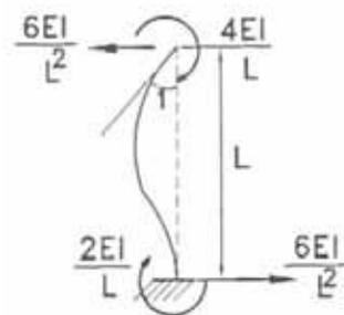
Fig. 1 Forces and moments generated ends due to unit rotation.
