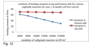
Variation of bending moment in top and bottom slab for various subgrade reactions for case 1 in double cell box culvert.
