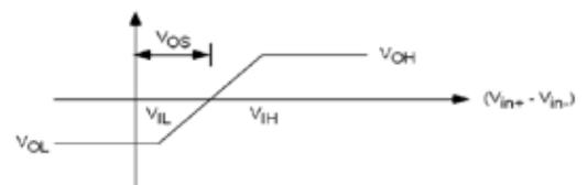
Figure 9 Transfer Characteristics of a comparator including
