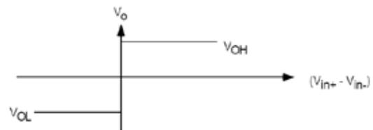
Figure 8 Ideal Comparator Transfer Characteristics
