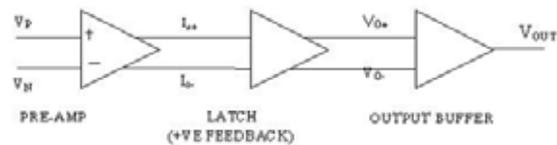
Fig.2 Block Diagram of High Speed Comparator.
