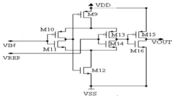
Fig. 5 Output Buffer of a Comparator
