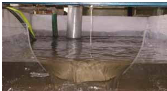
Figure 2. Weir evaluation experiment in hydraulic flume
