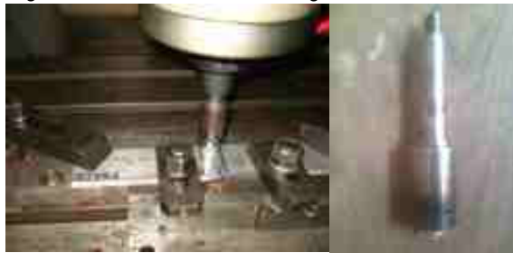
Fig.3 Tool used for friction stir welding
