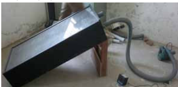
Figure 2.1 Working model of Solar air heater.
