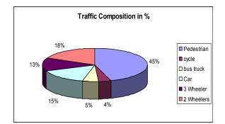
5.1.2 Radhanpur cross road: Traffic volume count survey conducted at morning 9:30-12:00 and evening 4:30-6:30 PM,total 4:30 hours survey carried out by supporter .below table following different components of traffic.
