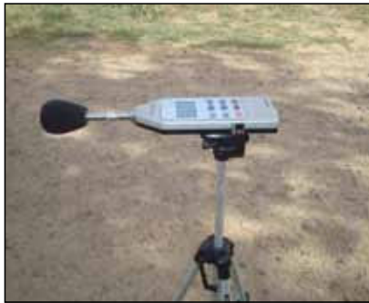
Fig-1.1 Sound level meter on a tripod with windscreen
