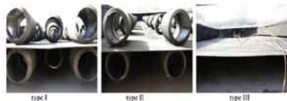
Figure 8: aluminum can as obstacle in double flow solar air heater [10]
