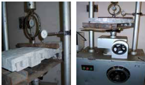
Figure 5: Experimental setup for flexural loading test Result and Analysis
