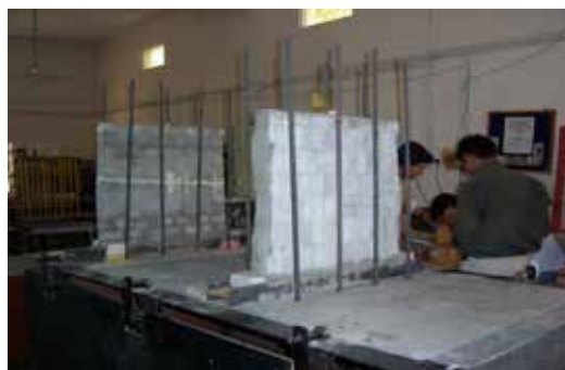
Figure 6: Experimental set up for Shake table testing.
