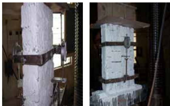
Figure 2: Experimental set up of compression test.
