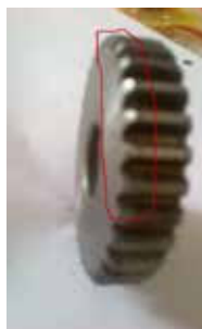
Figure 8 Improper chamfer defect
