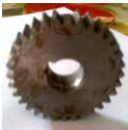
Figure 5 full tooth breakage defect
